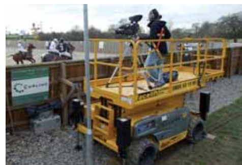
The Haulotte DX12 compact scissor RT scissor lifts made ideal camera stands.
