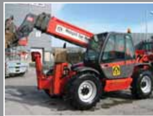
Manitou MT 1740 Telescopic forklift 17m/4 Tonne - 2005
