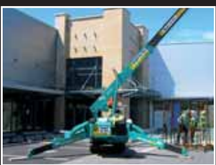
MAEDA MC405 CRM-E Mobile minicrane 16.8m - 3.8 Tonne - 2007
