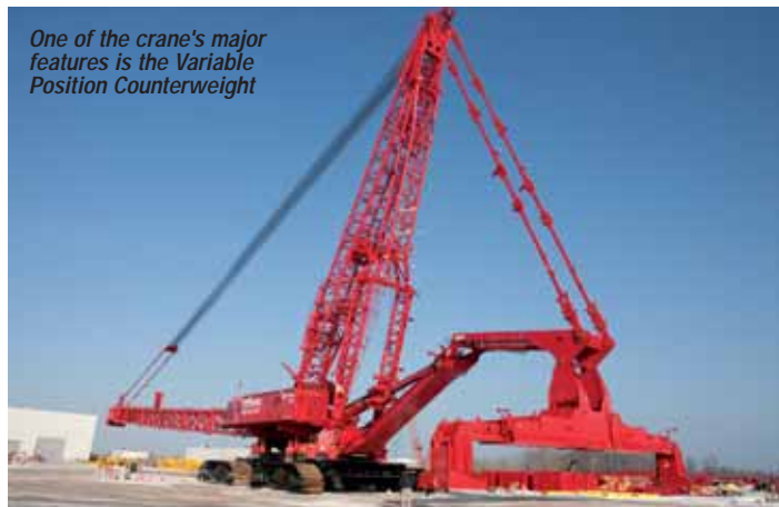
The counterweight always remains suspended saving customers time and money preparing the ground
