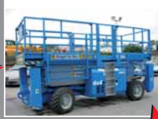
Genie GS-3384 RT Diesel scissor 12.06m - 2006
