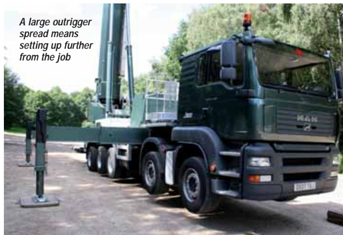
More manufacturers have models with outriggers within the width of the vehicle
