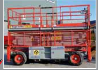
SkyJack SJ 9250 Diesel scissor 17.1m - 2007
