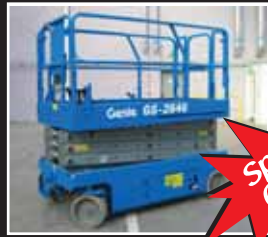
Genie GS-2646 Battery scissor 9.9m - 2004/5/6/7/8
