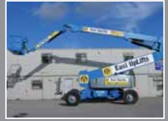
Genie Z-135/70 Articulated boom 43m - 2007/8
