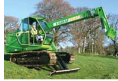
The Giraf Track with optional V blade slope levelling and anchoring system.
