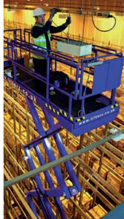
The 1.2 metre wide, 22.5 metre working height S225-12ES
