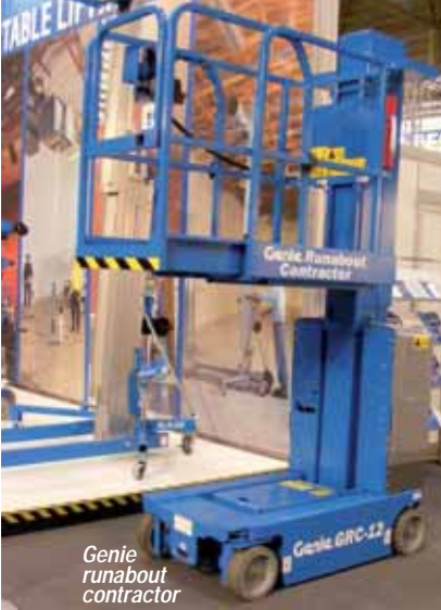
service access is excellent even with the platform lowered
