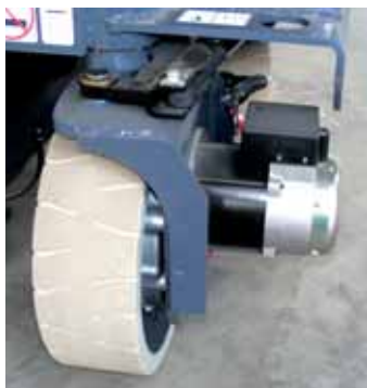
Aichi's new electric scissor lifts use AC wheel motors rather than DC.
