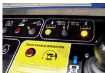
The Genie X system of platform capacity selection.
