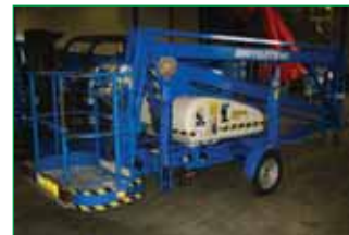
TRAILER MOUNTED PLATFORM 1999 Niftylift 140HDC 14m working height (46ft) Hydraulic Legs, DC Only
