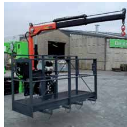
Glass panes and other heavy materials can be lifted by the 550kg telescopic overhead Palfinger lorry crane on this 2.5 metre long Giraf Track basket.
