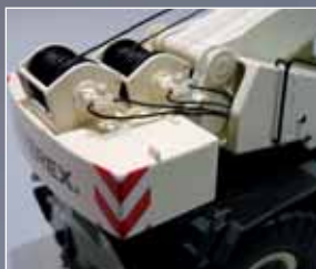
Hydraulic lines to the winches
