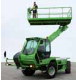
The MPR platform rotates 360 (2x180) degrees.
