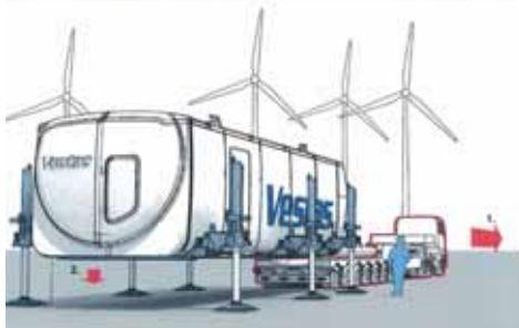
The blade transporter includes a sliding device that allows the combined overall length of tractor and trailer to be used.
