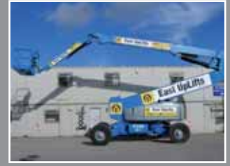
Genie Z-135/70 Articulated boom 43m - 2007/8
