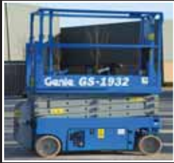
Genie GS-1932 Battery scissor 7.8m - 2004/5/6/7/8
