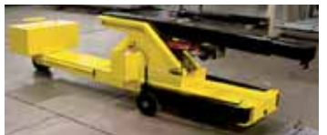
The counterweight tank extends for additional ballast effect.
