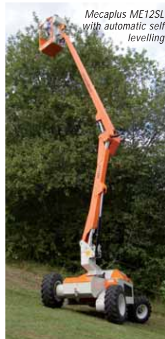
The ME12SL has 7.6 metres outreach, 340 degrees slew and 180 degrees basket rotation
