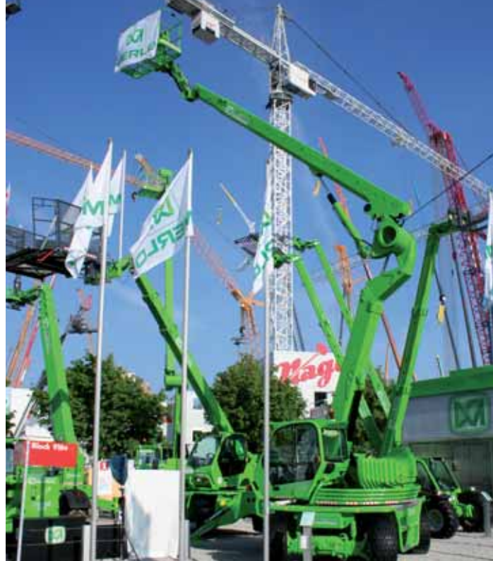
The most unexpected platform at the show - Merlo's MPR series combines a modified Roto telehandler chassis with an articulated telescopic boom.
