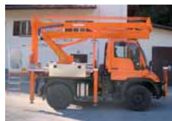
Mounted on a Unimog chassis, the Teccio 16 metre platform has a 'go anywhere' capability.
