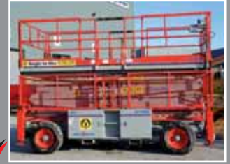
SkyJack SJ 9250 Diesel scissor 17.1m - 2007
