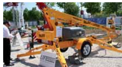
Bil-Jax is hoping for a sizeable slice of the market with its 13.4 metre working height T134/98.
