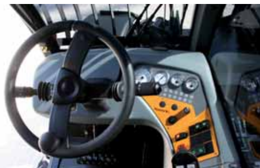
The new Haulotte dash features a single multi-function controller which allows one-handed operation.
