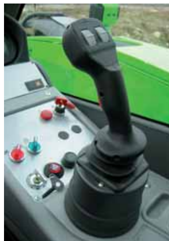
The new Merlo cab has a single joystick with electro-proportional controls.
