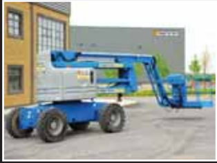
Genie Z-60/34 Articulated boom 20.4m - 2004/5/6/7/8
