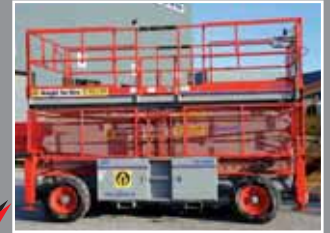
SkyJack SJ 9250 Diesel scissor 17.1m - 2007
