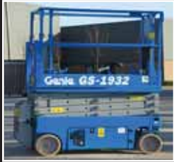
Genie GS-1932 Battery scissor 7.8m - 2004/5/6/7/8
