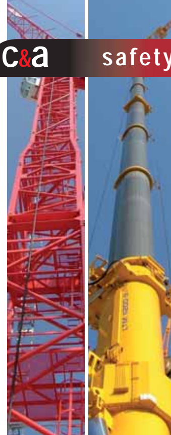
When putting very high booms into the air there might be restrictions as far as 15km from an airfield.
