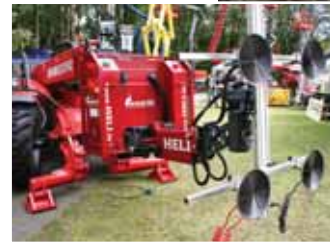
The Guerenuk 500 telehandler mounted glass handler on the Heli stand.
