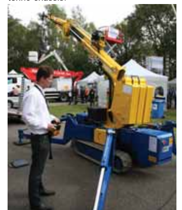
There were several tracked mini cranes including this 17.4 metre reach, 4 tonne maximum Hoeflon C610.
