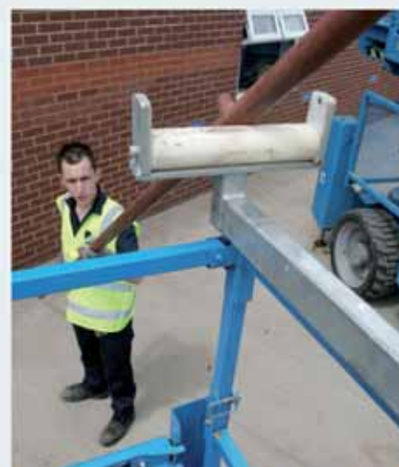
Lavendon offers a range of material handling attachments for scissor and boom lifts enabling the quick and safe installation of materials (up to 600kg) of varying lengths.
