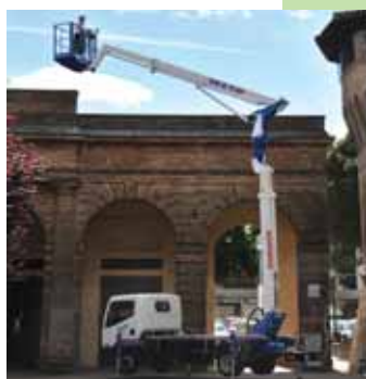
CTE launches its radical new 20.13MP truck mounted lift with slew ring mounted on top of its two-section lower boom.
