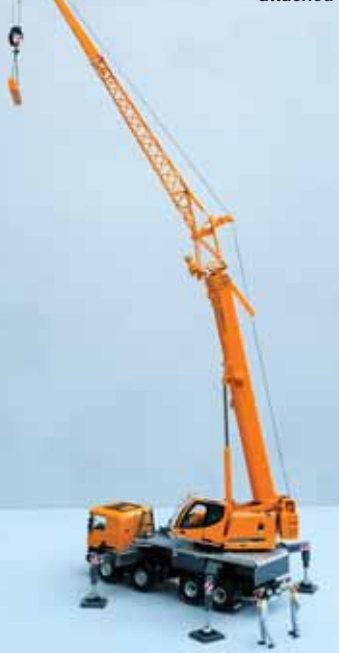
Swingaway boom extension attached
