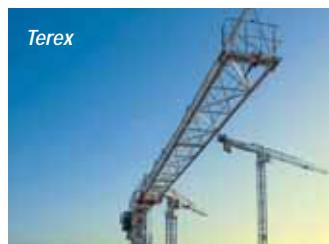
past JCB and onto the Terex stand to see another hammer-head - the 20 tonne Comedil Terex SK 415-20 tower crane. Equipped with the new EVO15 cab and new longer 80 metre/264ft jib at which radius the crane can handle 2.3 tonnes. A new HD23-TS212 transfer mast is available, which provides a free standing height of 91.6 metres/300ft. Last stop on this tour is to cross the main Lot to the Silver Lot to see Zoomlion.
