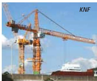
be completely pre-assembled including the moveable cab, switchgear cabinet, jib folding frame, slewing gear, slew ring and support and the current collector. Jib lengths are available up to 75
