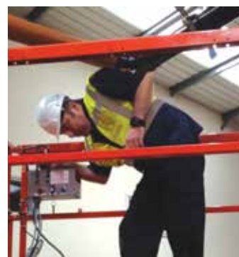
The idea is that if an operator is pushed down on the controller his forearm will activate the system.
