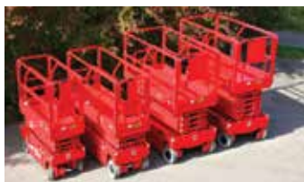
PB's compact 14 metre model (L) has an excellent specification and is the narrowest at 1.15 metres, and one of the lightest at 2,910kg.
