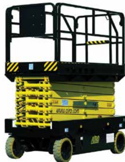
Airo's 14m X14EW has a 1,500mm deck extension but weighs 3,365kg.
