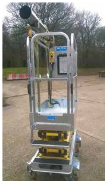
The DRXmicro can support loads up to 40kg.
