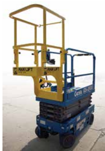
US-based Manlift Manufacturing offers the SHU-30 attachment that can be swapped with a standard roll-out deck extension on a 19ft Genie GS1930, to offer a 750mm step up (Single Hop Up-30inch) for use to gain access through false ceiling panels etc.
