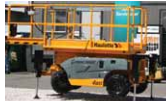
Haulotte Compact 2668RT - 4WD, 40% gradeability and 47 inch platform extension
