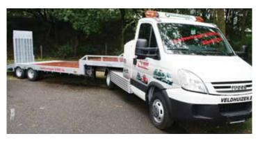
of axle weights and the emergence of trailers with more axles. Heavy equipment hauliers across Europe are now increasingly using more four axle trailers, although three axle units still serve most requirements within the regular 44 tonne weight limit.
