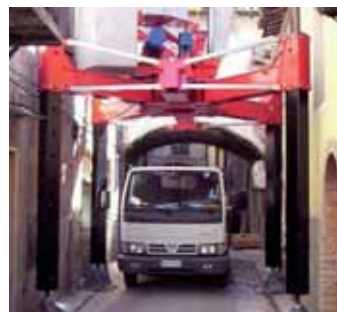
Clever Crane's telescopic chassis allows up to 2.75 metres of head height giving access to cars and pedestrians.
