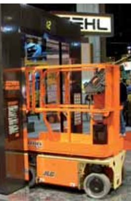
The new JLG 1230ES demonstrating its ability to ride elevators
