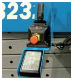
The Controller has an extra pad for setting the outriggers.
