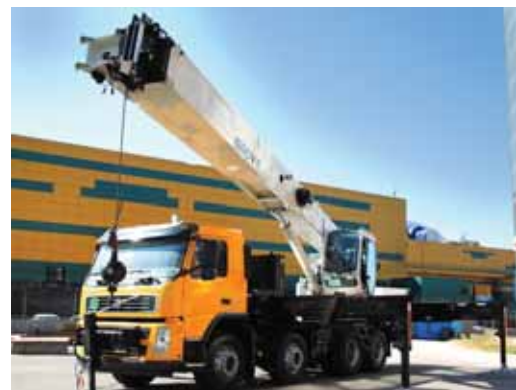
The Grove GBT35 truck crane has a 35 tonne capacity and 39 metre five section full-power boom.
