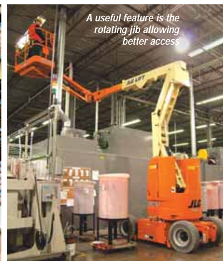
Checking cabling at a chemical plant using a mast boom
