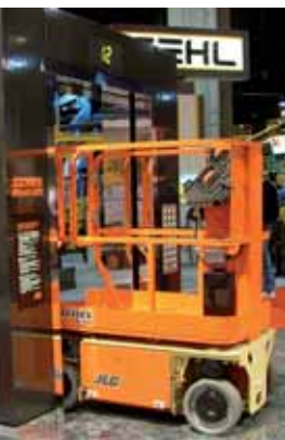
The new JLG 1230ES demonstrating its ability to ride elevators
