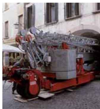
When folded, self erectors are small enough to gain access through some surprisingly small openings.
