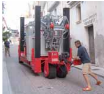
The Gelco Clever Crane's 4WD chassis can cope with gradients up to 25 degrees..
