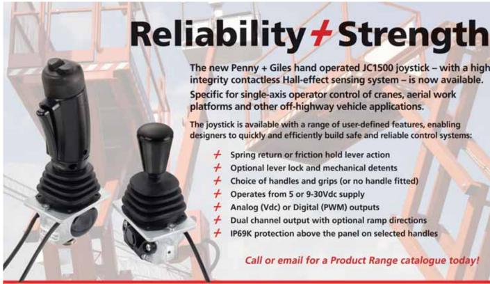
The new Penny + Giles hand operated JC1500 joystick - with a high integrity contactless Hall-effect sensing system - is now available.
