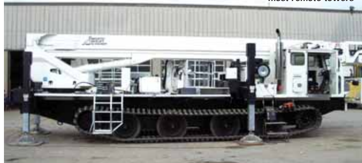
A 47 metre Bronto insulated lift on special tracked carrier can reach all but the most remote towers
