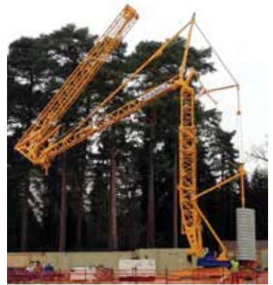
With an under hook height of 20 to 35 metres the T85A can handle up to 1,400kg to a radius of 45 metres.
