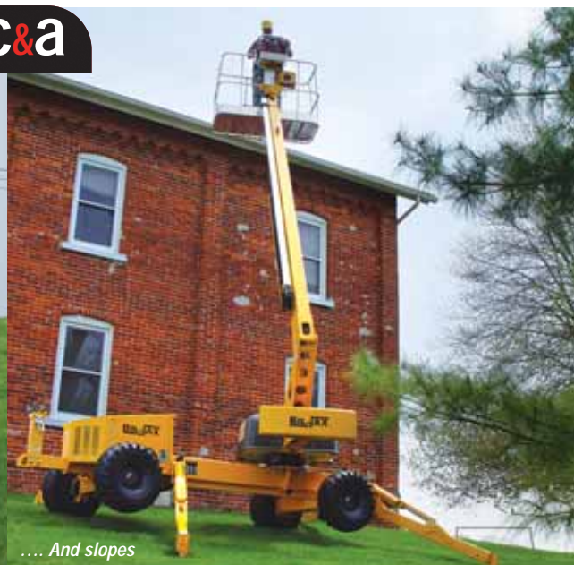
The Bil-Jax 36XT demonstrates how this type of lift easily copes with soft ground....
