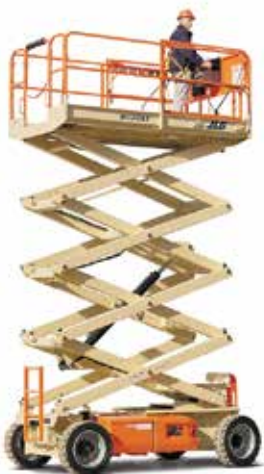
The JLG M3369LE uses two DC electric wheel motors and 4.5kW Kubota diesel charging the battery pack.
