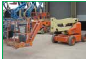
SELF PROPELLED TELESCOPIC 2001 JLG M45J. 15.5m working height (51ft). Fly Jib, Bi-Energy.
