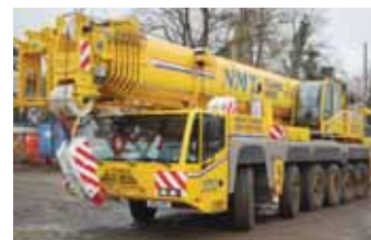
NMT's new six axle Terex AC200-1P can travel with up to 25 tonnes of counterweight along with all its tackle and steel outrigger mats.
