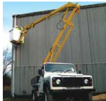
A Gardner Denver Land Rover mounted lift.
