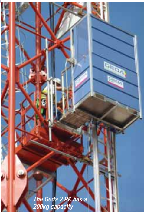
For erection lightweight aluminium ladder sections are passed through the open car roof and fixed using the patented quick-lock system
