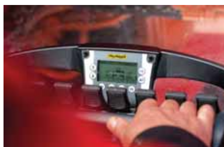
Both main control station and remote controller displays show percentage of extension for each outrigger
