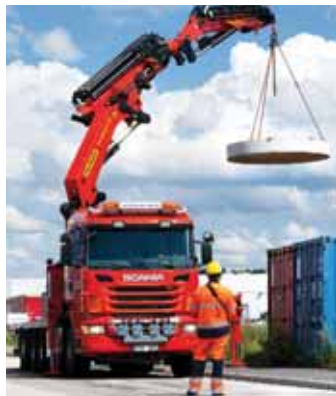
Palfinger's new HPSC system automatically adjusts the cranes working envelope and lift capacity according to outrigger set up and is being fitted across the range
