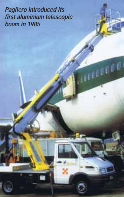
Pagliari was always innovative, its big booms use gearboxes to rotate its jibs as well as allow some unique configurations
