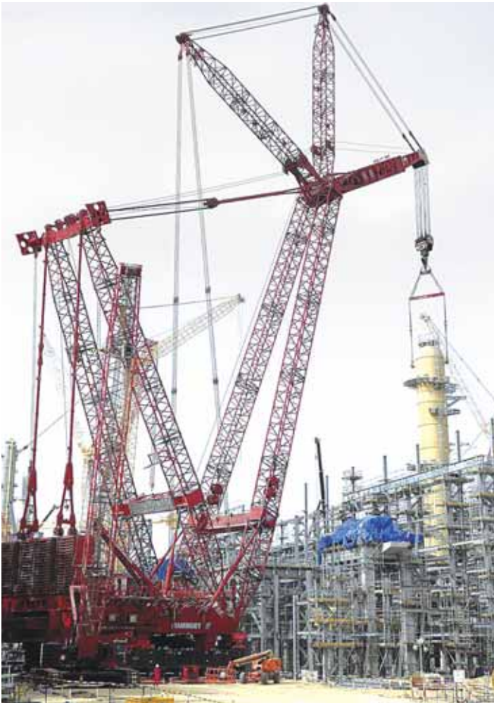
Mammoet has been building PTC cranes since 1996 - here is a PTC 1 in a petrochemical application lifting 670 tonnes.
