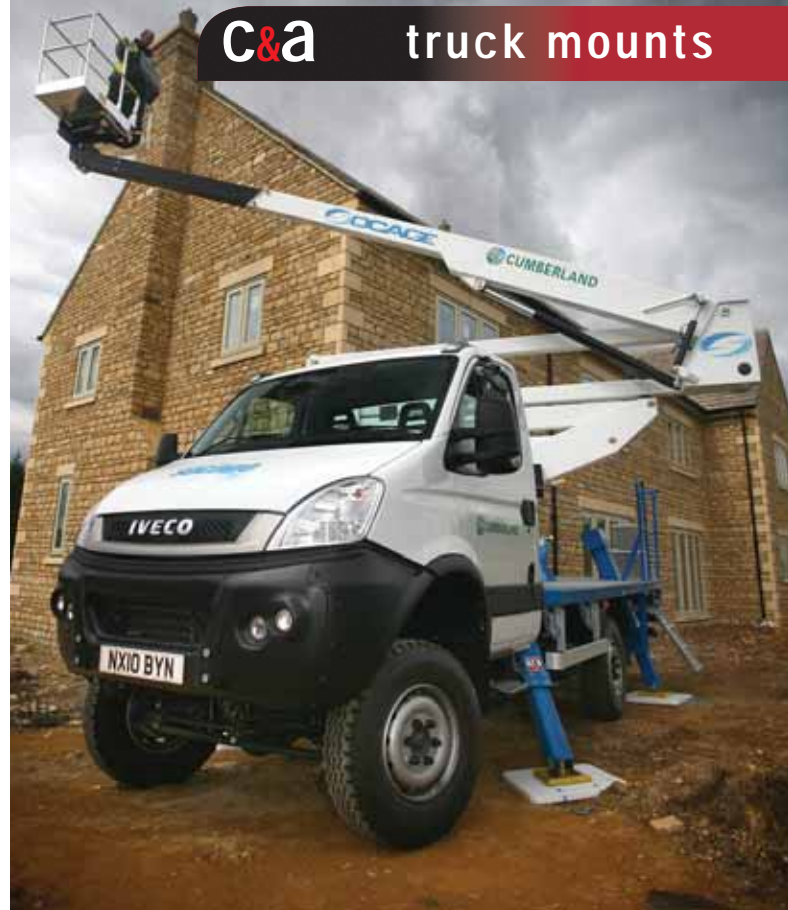
The older Z20E has 200kg basket capacity and A frame outriggers
