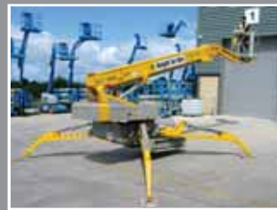
OMME 3000RBD Specialised boom 30m - 2006/7/8
