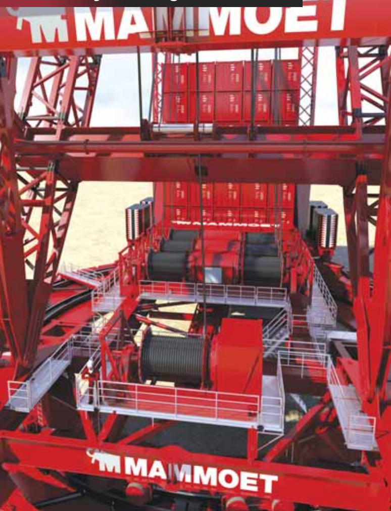
The PTC has four 800 tonne high speed main winch systems.
