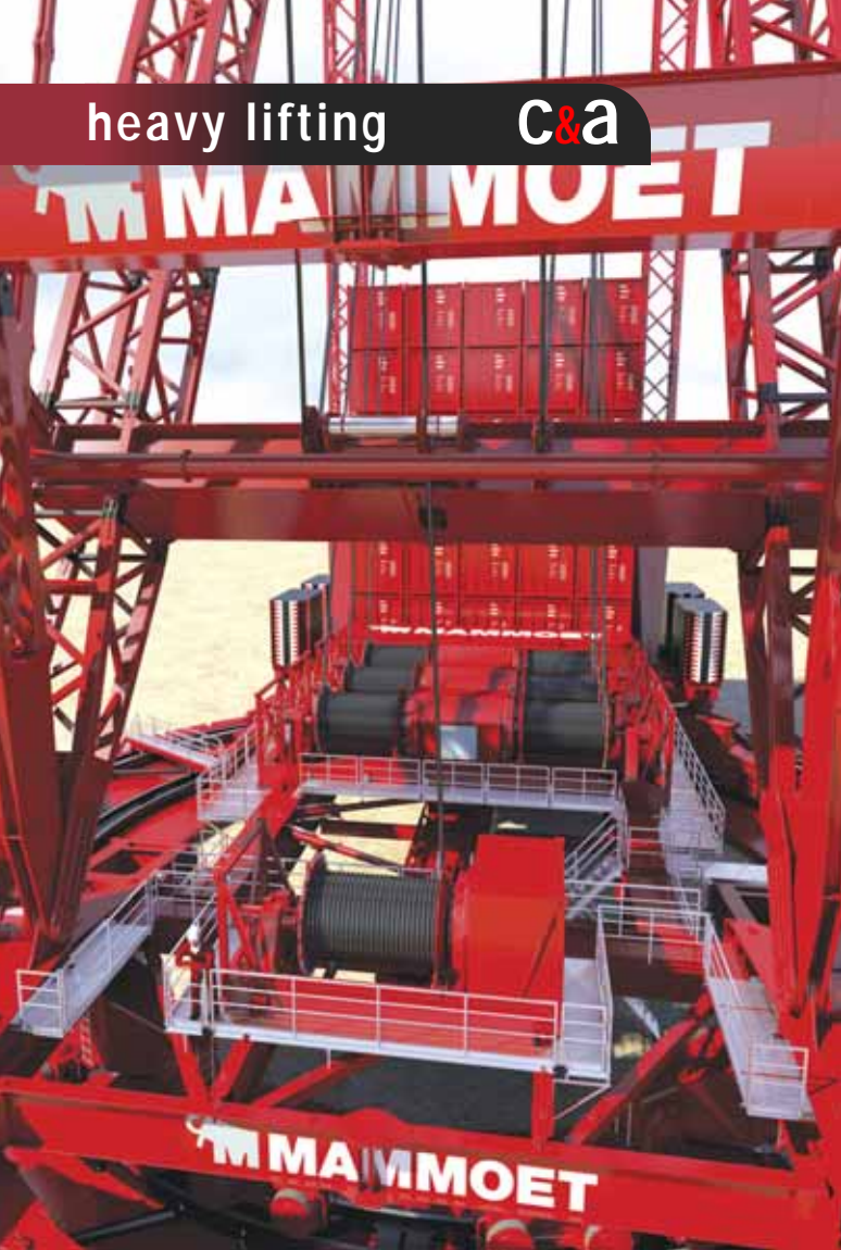
The PTC has four 800 tonne high speed main winch systems.
