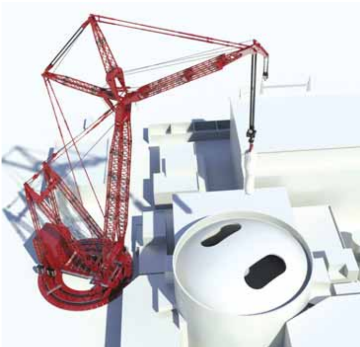
Mammoet says its new generation PTC's are 'real' cranes, not sliding gantries or lifting machines.
