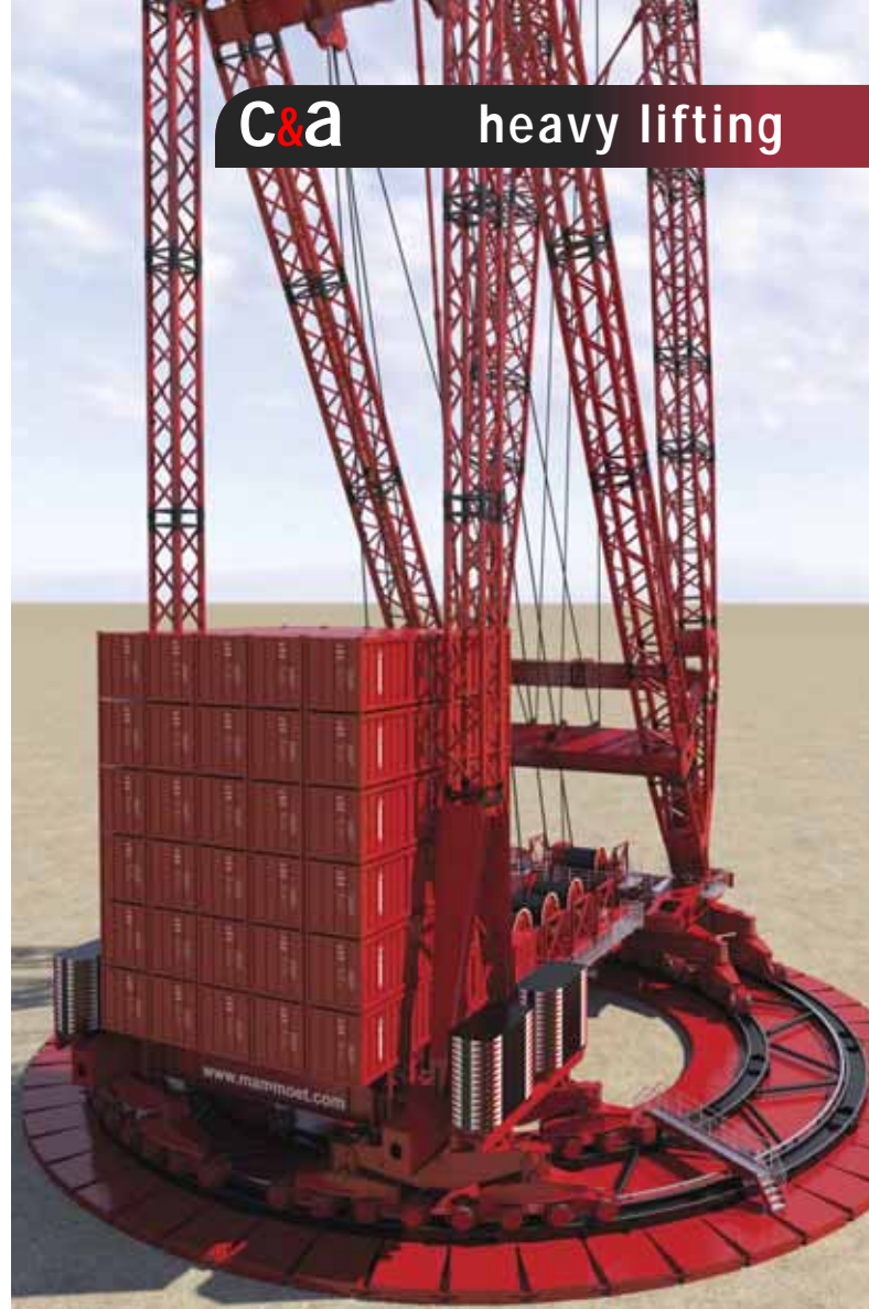
Ground bearing pressure is 20 tonnes per square metre (4,100/sqft) for both cranes and is combined with a relatively small footprint (45 metres and 55 metres).
