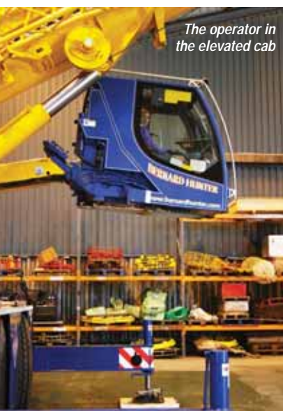
Elevating the cab on the LTC 1045 gives the operator a vastly improved view of the lift
