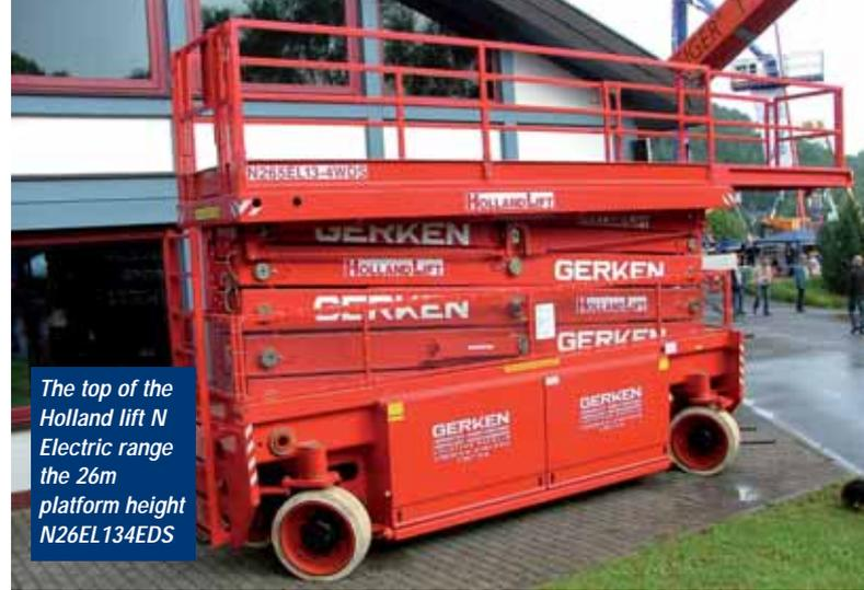
*The top of the Holland lift N Electric range the 26m platform height N26EL134EDS*
