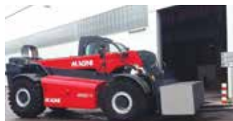
The first Magni in the steel industry - an HTH 27.11 - is ideal for handling heavy ingots.
