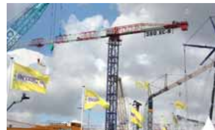
The new 380 EC-B 16 Litronic flat top crane rated at 380 tonne metres its Liebherr's largest in the 15 model range.
