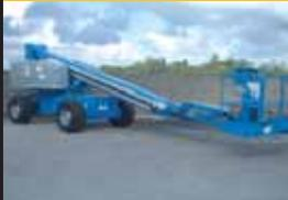
Spec: 4WD telescopic boom. Deutz diesel. 91ft work height (27.7m) Choice
