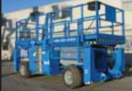
Spec: 4wd Kubota diesel scissors, 39ft work height (12m) Deck extension, hyd. Outriggers, choice
