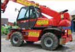
Spec: 4wd rotator, 21m work height. 5 tonne capacity. Hydraulic jacks. 3tonne Winch and operator basket
