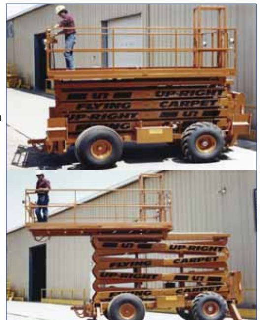
This rough terrain UpRight Flying Carpet of the early 70s has a platform height of 47ft with a 6ft hydraulic cantilever platform and a dual fuel petrol/propane system. Other features included a tow bar, 120psi and 120V power to the platform, spark arrestor exhaust system and foam filled tyres.
