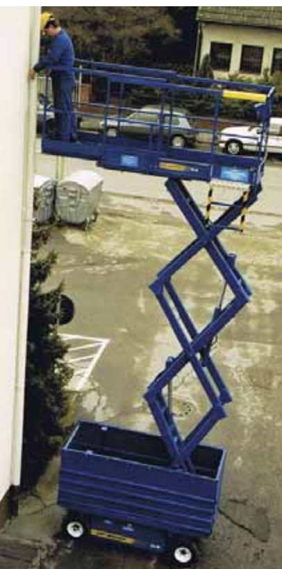
The idea of an electric scissor lift that can handle gravel and softer ground has been around for more than two decades - one such machine was the UpRight XL24 from the late 80s and early 90s.
