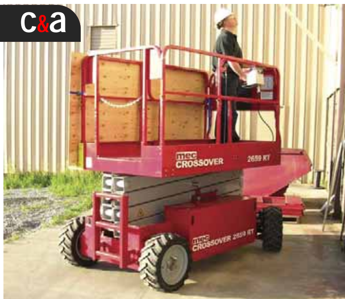
The Mec Crossover is available with a 26 or 32ft platform height - both with an overall width of 59 inches (1,499mm) so they will pass easily through a set of double doors.
