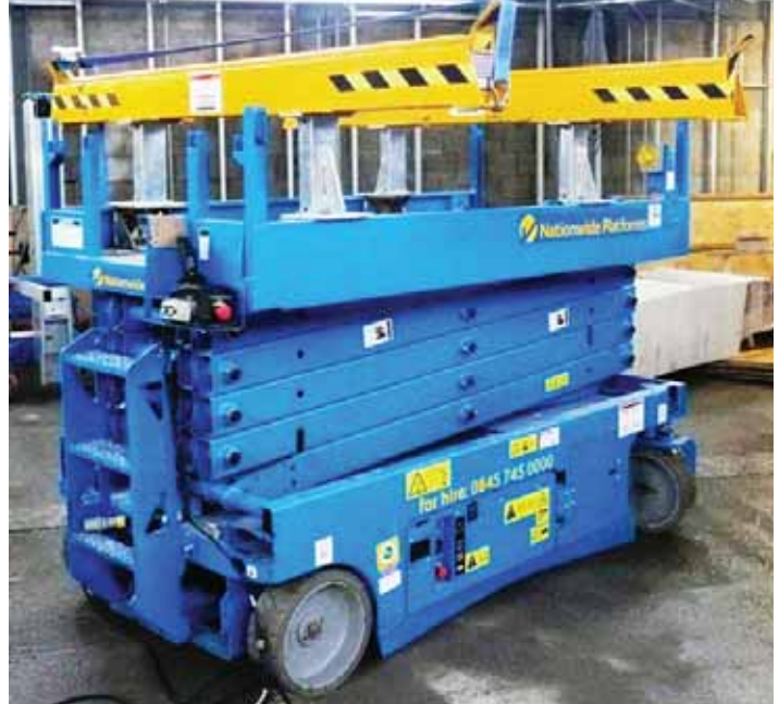
Nationwide Platforms supplied this SkyDuct attachment fitted to a modified Genie GS2646 scissor lift, capable of holding up to 350kg of materials without risk to operators or materials falling to the ground.
