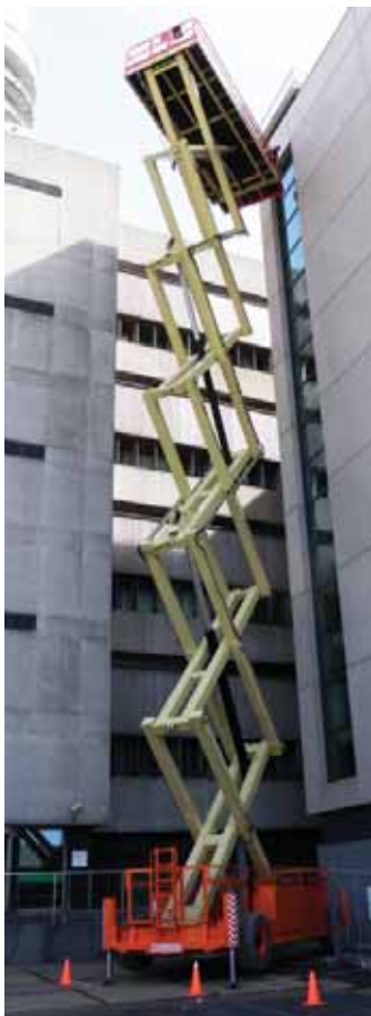
Holland Lift's massive, electric 33.7 metre working height Megastar G-320DL30 4WDS/N.
